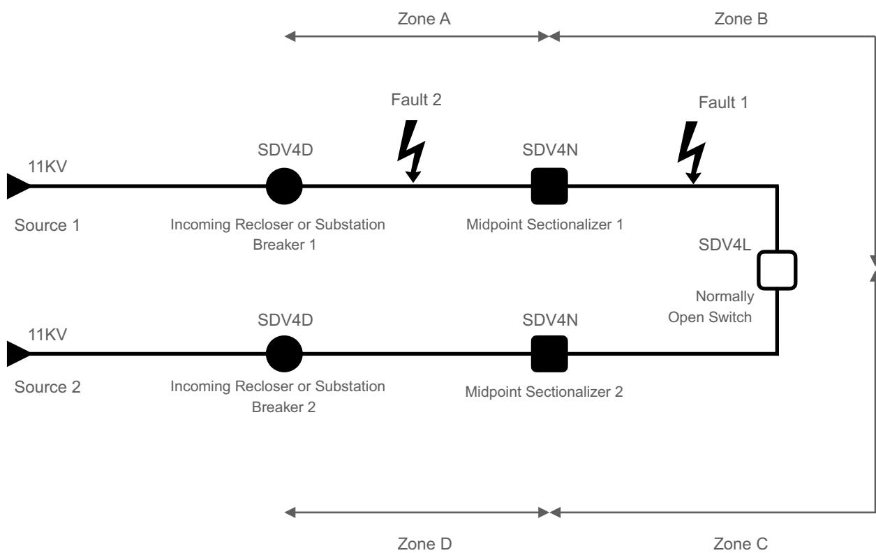
A practical application of the Sectionalizer is illustrated in the diagram above. Two feeders (Feeder 1 and Feeder 2) are connected through a Sectionalizer, which is typically in the open condition, with voltage sensing on both the incoming and outgoing sides. Reclosers handle fault interruption, while the Sectionalizer is positioned at a midpoint for fault isolation. Two case scenarios are described below for clarity:
